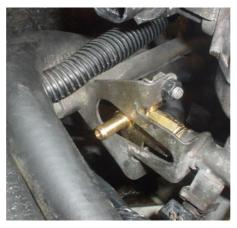
You should use the two bolts that were removed earlier to secure this in place.
