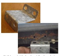
At this point I also bent the bracket ready for the Power boost valve to be fixed to it. As seen above.
