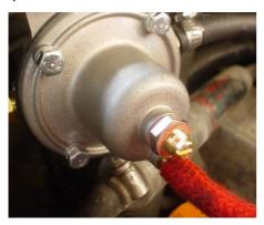
Now loosen then second nut that is on the adjustment screw.
