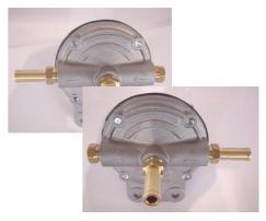
The input pipe is the one coming from the side of the Power boost valve and is going to be connected to the adaptor plate. As you can see I have had to change my one for this Range Rover from one side to the other.
