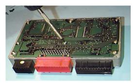
The circuit board itself may then be released by unscrewing the 8 screws that hold it in place, using the picture for assistance.
