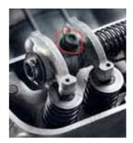
To insert the shims, you need to slacken all 8 of the 14mm bolts that hold the rocker pedestals in place.
