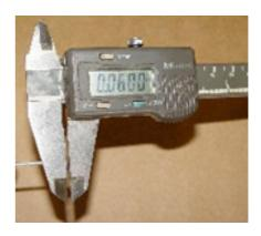
There are currently no tools available for measuring this gap. However, we have found that the best item to use is a length of welding rod with one end bent at 90 degrees. You will need a measuring device, such as the vernier shown, to select/create 2 welding rods; one that measures at 40 thou., and the other that measures 60 thou. in diameter. This will give you an idea as to what shims you need to fit under the pedestals to set the pre-load.
