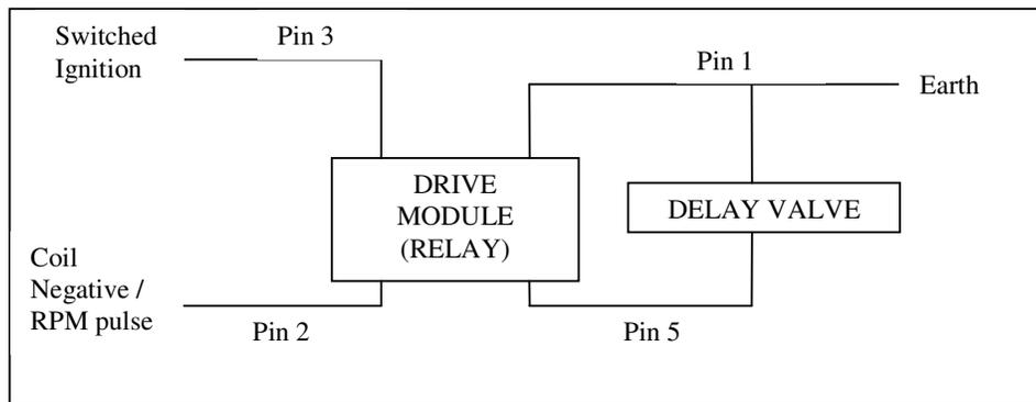
The **Delay Valve** (the black unit fitted between the SU carb. and FASD unit) only has two connections, one connection is connected to the output of the Blue DRC 8039 FASD **Drive Module** (Pin 5) and the other terminal is connected to an engine or chassis earth.
