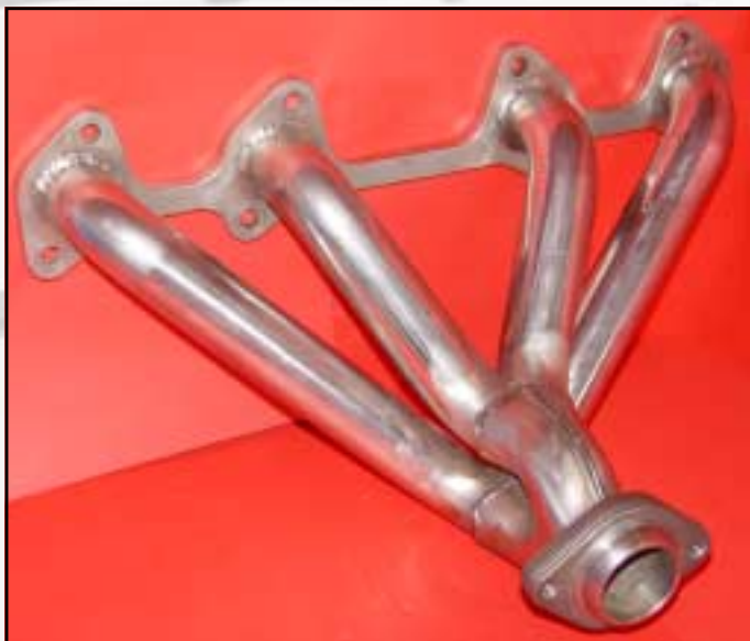
RPI +8 Manifold. Mandrel bent 304 grade Pictures shown also have Camcoat treatment inside and out.
